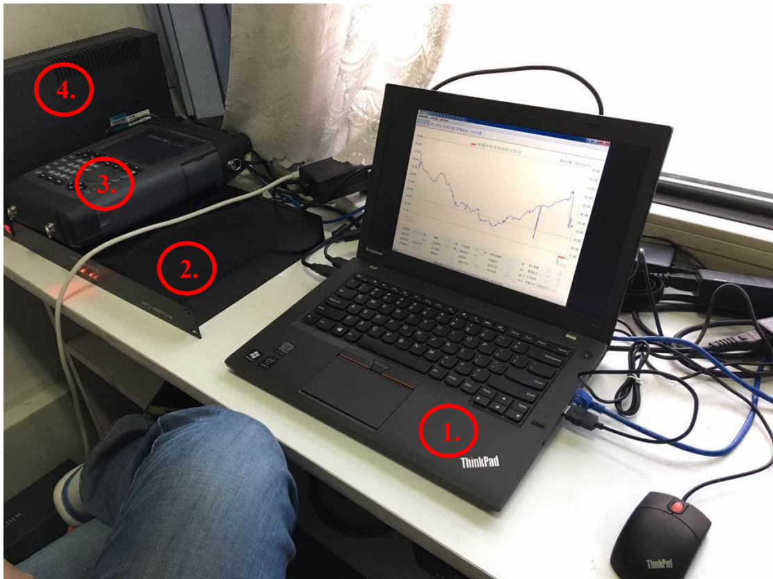
Fig.2 the FST system include (1) Host Computer, (2) Sensor Adapter, (3) PR100 Wireless Strength Test Device, and (4) UPS.
